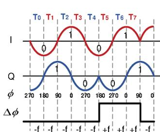
Fig. 8: The phase shift of OQPSK signals
