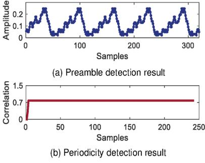
Fig. 4: The detection result of ZigBee preamble and the periodicity detection result
