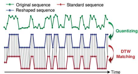
Fig. 10: Matching filter based decoding
