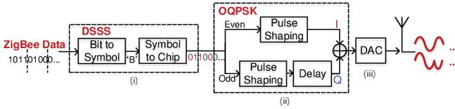
Fig. 1: The workflow of a ZigBee transmitter
