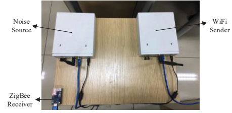
Fig. 16. The experiment platform: a prototype of WiZig, one USRP acts as WiFi sender, another USRP generates Gaussian noise and TelosB mote is used as ZigBee device
