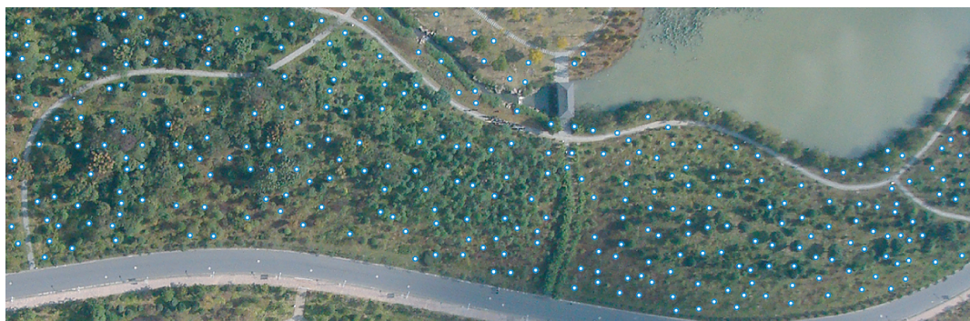
Fig. 2 Bird's-eye picture of a GreenOrbs prototype (each blue point denotes a sensor node)
