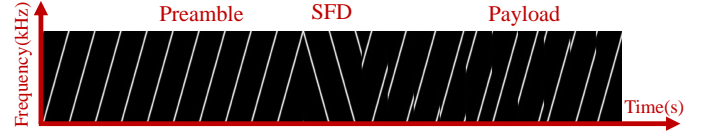
Fig. 2. LoRa packet structure.
