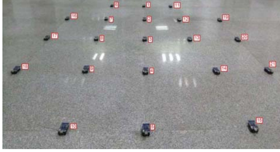
Fig. 7. Checking the propose approach on a testbed of 21 TelosB motes
