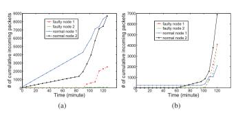
Fig. 13: Incoming packets for QoF and ETX in case II. (a) CTP-QoF, (b) CTP-ETX.
