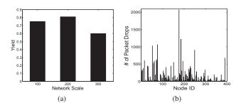
Fig. 2: Observation from a 330-node outdoor test-bed. (a) Network yield at different scales. (b) Packet loss on different nodes.
