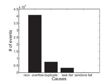
Fig. 5: Different causes of packet loss on sensor nodes.
