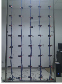
Fig. 16. The picture of real testbed with 50 TelosB nodes.
