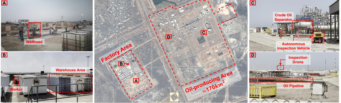
Figure 1: Industrial inspection is carried out by 10 drones and 2 autonomous vehicles in a large oil-field. These agents are coordinated by SwarmMap that runs on an Nvidia AGX Xavier edge server.
