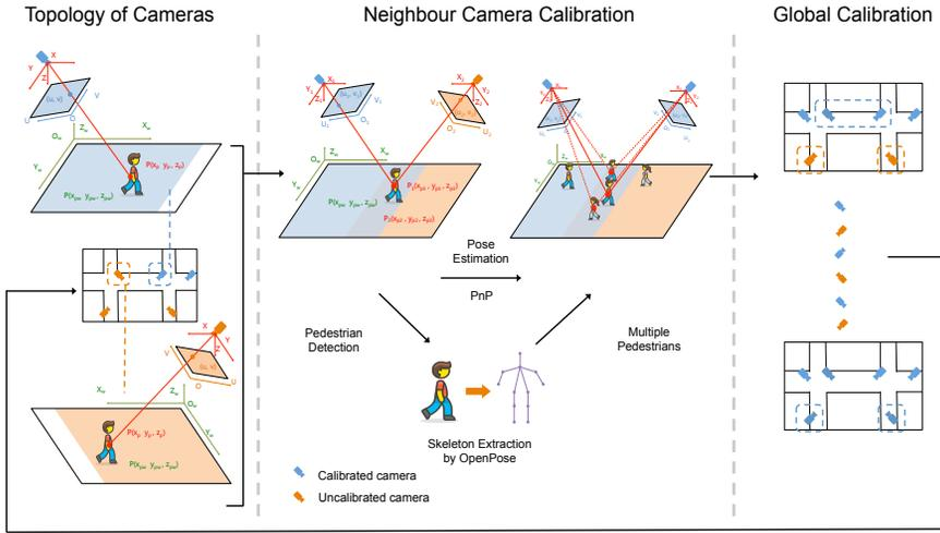
Fig. 4. Workflow of Automatic Camera Calibration
