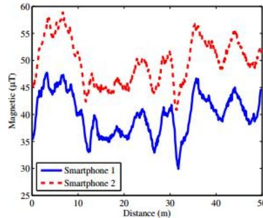
Figure 2. Magnetic readings captured by two smartphones along a 50-meter corridor.
