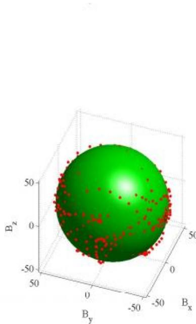
Figure 1. Locus of magnetic readings with the optimum ellipsoidal fit superimposed.
