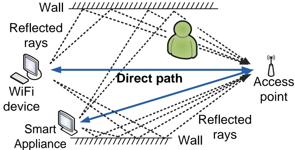
**Reality: Large Localization Error** roots in rich Multi Path Propagation Indoors
