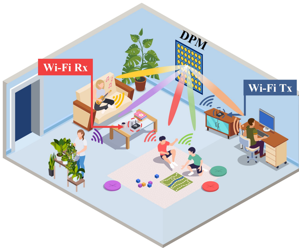
Fig. 1. Typical application scenarios of multi-person respiration detection based on DPM-aided Wi-Fi. The DPM works with Wi-Fi terminal to separate and detect breathing information from multiple people in the same space using time and space modulation capabilities.
