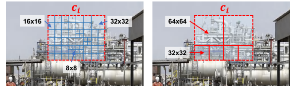
(b) A comparison of block-level division results between a standard codec (left) and E-Cube-integrated codec (right)
