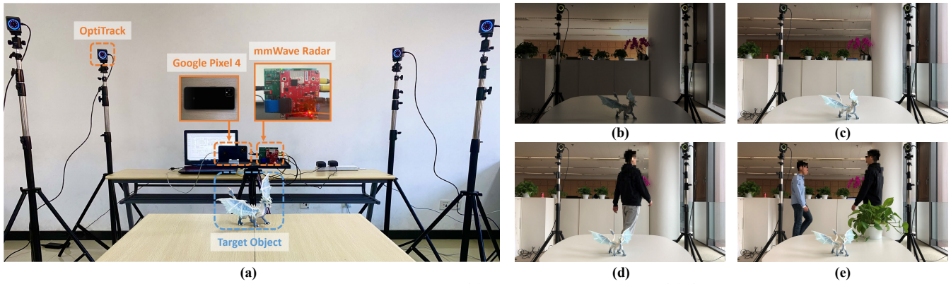
Figure 7: Experimental setup and scenarios of FollowUpAR. (a) A laboratory scenario. (b)-(e) A crowded office with different illumination intensity (normal and weak), as well as diverse background dynamics (static, slight, and severe), respectively.
