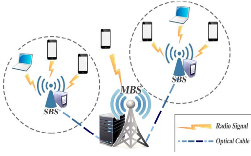
Fig. 1. MEC system in 5G networks
