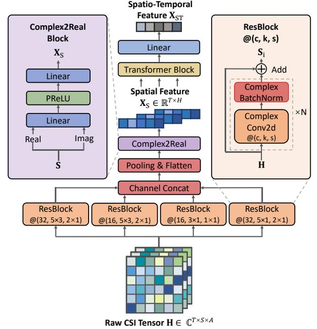
Fig. 3. Illustration of Multi-Resolution Spatio-Temporal Encoder.
