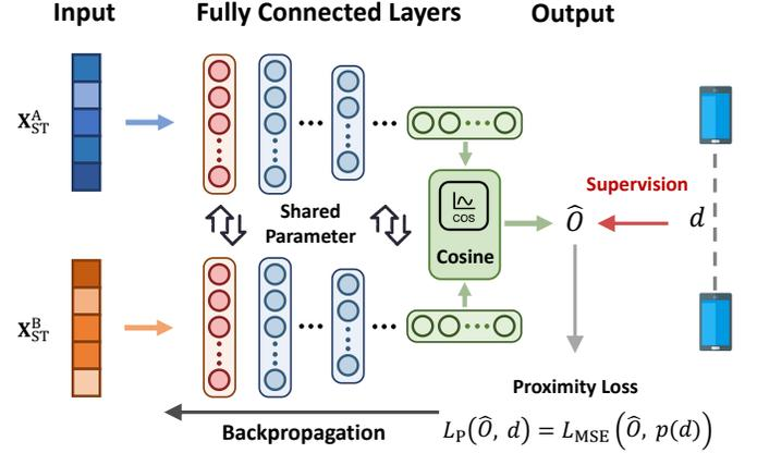
Fig. 4. An overview of the Proximity Metric Adaptation Network.
