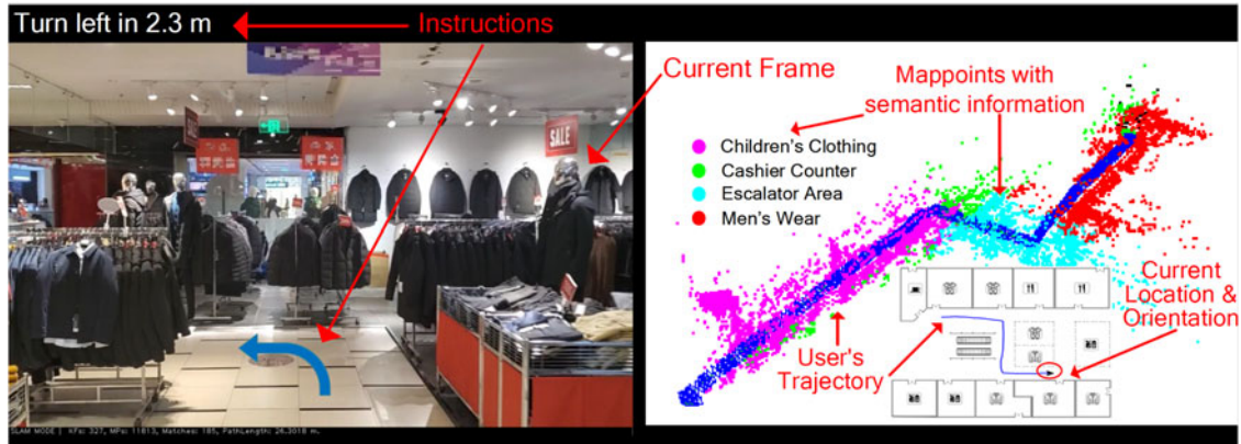
Fig. 1. User interface of our navigation system. iSAT provides users with: 1) instant location and orientation in constructed map and floorplan, 2) navigation instruction rendered in user's view and distance to next crossing point, 3) semantic information about surrounding environment.
